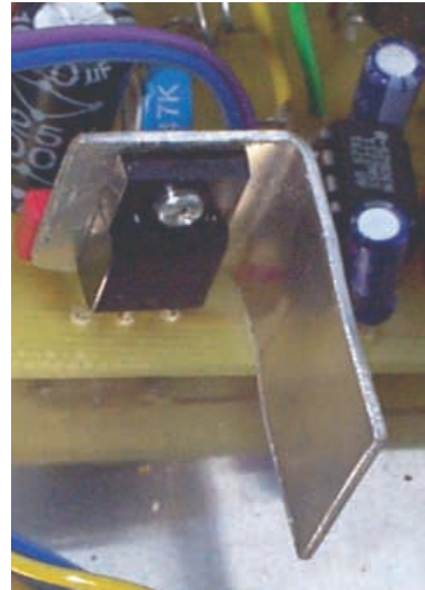
Close-up detail of heatsink mounted on IC3.
